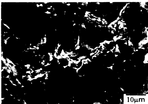
Fig. 10. Fracture surfaces of 650°C tempered HY-130 steels failed by SSRT in sea water+0.1N H 2 SO 4 +1g/L thiourea under -1.6 mA/cm 2 .
