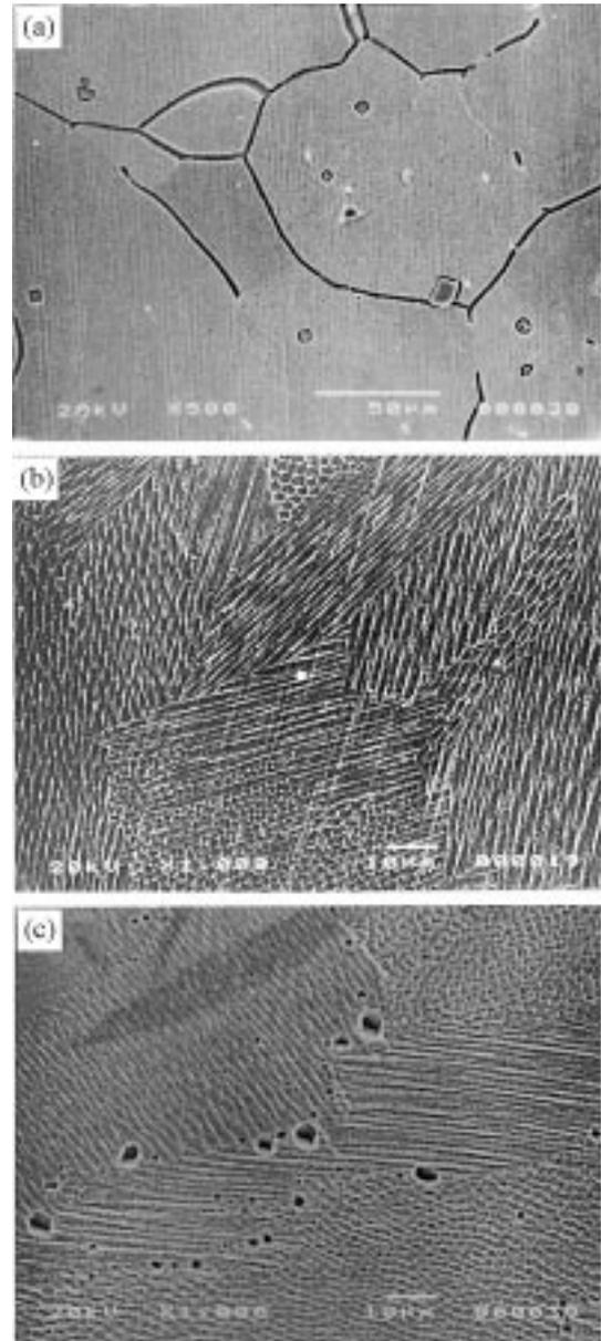
**Fig. 3.** SEM micrographs showing the surface morphologies after DL-EPT test for (a) the SA+SEN Alloy 600, (b) the LSM Alloy 600, and (c) the LSM+SEN Alloy 600, in 0.01 M  $H_2SO_4$ +20 ppm KSCN solution at a scan rate of 0.5 mV/sec at room temperature.
