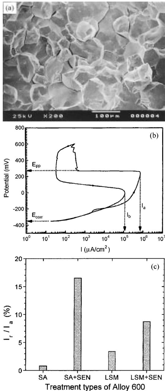
**Fig. 1.** (a) Fracture surface of the SA+SEN Alloy 600 after C-ring test, (b) a typical DL-EPR curve, and (c) DOS measured from the differently treated Alloy 600. (b) and (c) were obtained in 0.01 M  $\text{H}_2\text{SO}_4$  +20 ppm KSCN solution at a scan rate of 0.5 mV/sec at room temperature.
