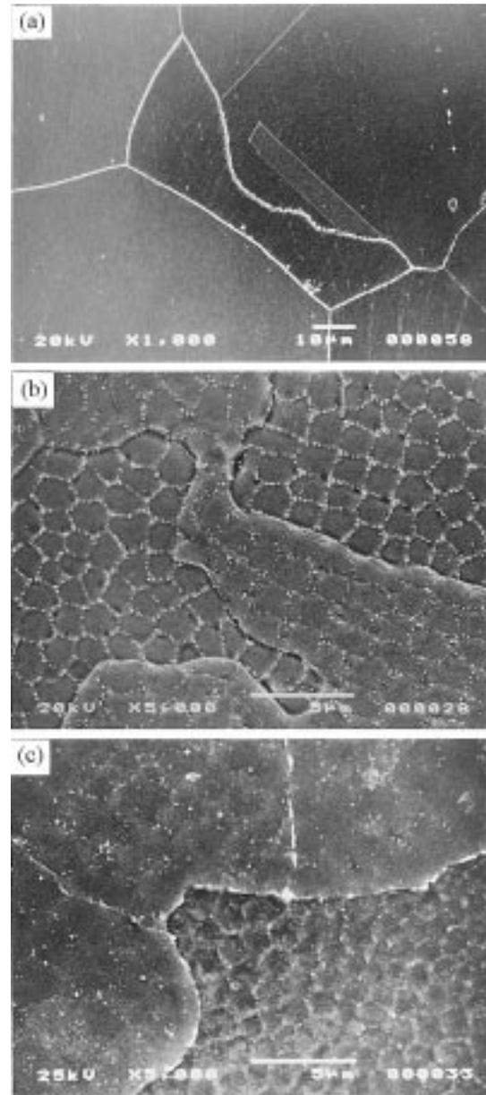
**Fig. 2.** Typical microstructures of (a) the SA+SEN Alloy 600, (b) the LSM Alloy 600, and (c) the LSM+SEN Alloy 600, etched in a solution of 2% HCl and 98% methanol.
